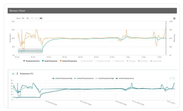
Comparison of temperature data from a live shipment in the Envirotainer Portal (top) and DB Schenker's IoT system (bottom)
